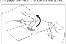
Ensure that the paper-foil layer is completely removed from the area over tablet.
